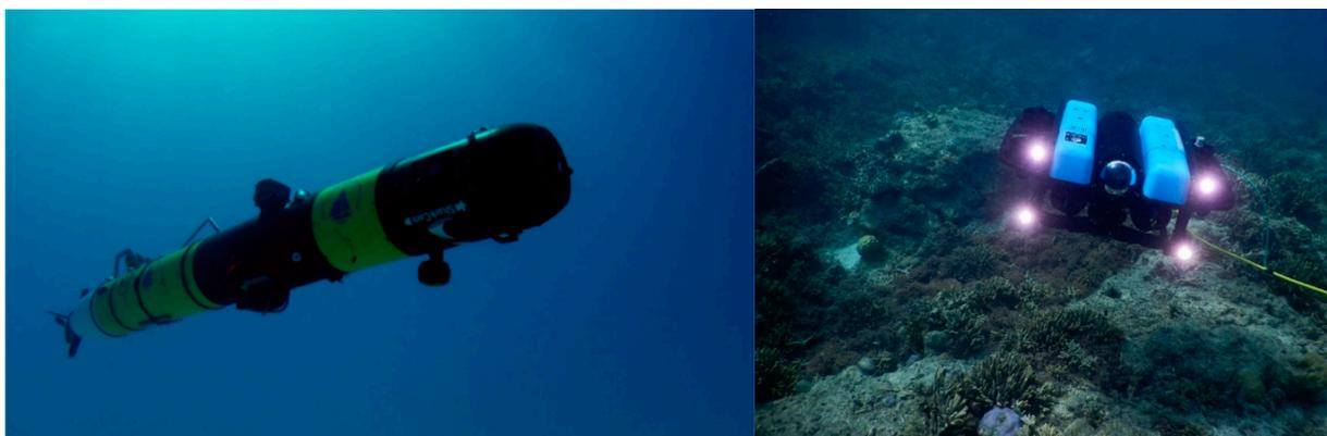
**Figure 6.** Examples of ‘underwater drones’ used for shark research. REMUS Automated Underwater Vehicle (AUV) used to track acoustically-tagged white sharks (*Carcharodon carcharias*) (left: Image—G Skomal), and BlueRobotics BlueROV2, a tethered, manually controlled remotely operated vehicle used to track untagged sharks post release (right: Image—T Gaston).
